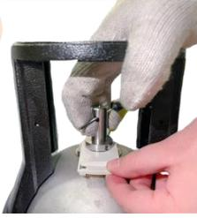
Lift up the pump shaft (#27) and plug in the mechanical seal spacer 'gasket'.
