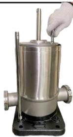
Install the four stay bolts (#47). Do not expose thread from the base plate more than 2 mm
