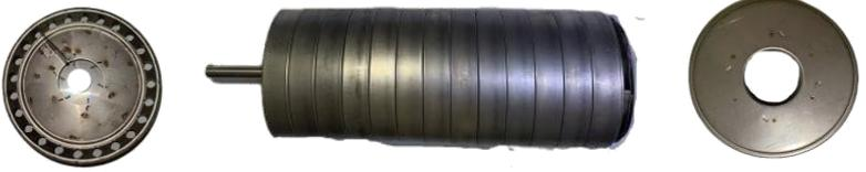
7 Note that the top diffuser (#7) and the inducer (#14) need to be inserted when assembling the pump body. The top diffuser (#7) is placed on top (left side), and the inducer (#14) is placed on the bottom (right side)
