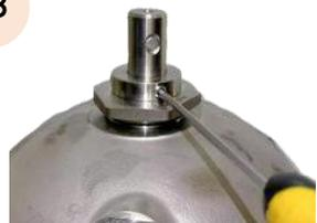
Tighten the three locating grub screws at the top of the mech seal (#8)
