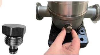
Place O-rings (#25 & #73) onto the drainage plug (#74) as shown. Install the drainage nut (#74) into the inlet / outlet chamber (#60) and tighten
