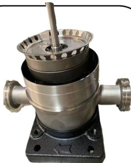
Fit the stack by lowering it into the inlet / outlet chamber (#60)
