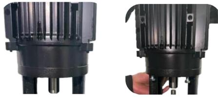
Use a lifting device to lift the motor (#32) and place it on the bracket (#63). Tighten motor retaining bolts
