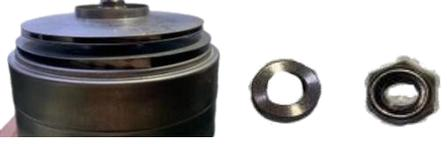
5 After placing the last impeller, install the inlet impeller cover (#19) and tighten the nut (#20)
