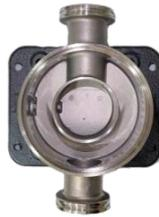
Install the inlet / outlet chamber (#5) on base plate (#10).
