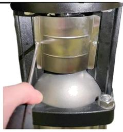
Install the coupling guard (#52) on the bracket (#63) and tighten the screws (#53)
