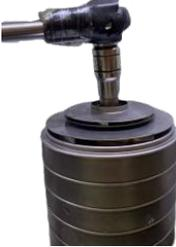
6 Tighten the nut (#20) with a torque wrench  $45 \pm 5$  Nm
