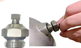
Place O-ring (#25) on air vent nut (#6). Install the air vent nut (#6) and tighten it
