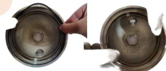
Install spring (#56) into seal base (#30). Edges of spring must point downward as shown for all models. Place O-ring (#24) into recessed area of seal base with some oil.
