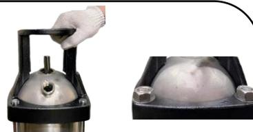
Seat the bracket (#63). Fit washers (#45) and nuts (#22) on the four stay bolts (#47) and tighten them.
