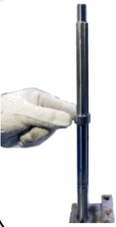
1 Fit the shaft (#27) into the shaft holding jig. Press the locating sleeve (#58) onto the shaft, and down onto the locating circlip.
