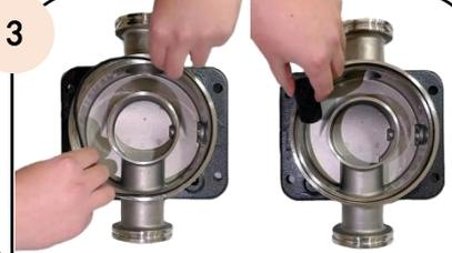
Spray vegetable oil on to the inlet / outlet chamber (#10) and O-ring (#24). Stretch and place the O-ring into the inlet / outlet chamber (#10) recess
