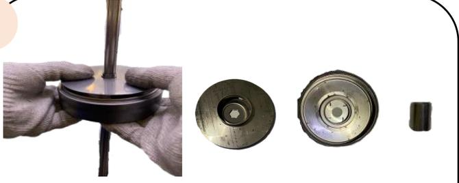
2 Install the impeller (#36), diffuser (#11) and impeller sleeve (#16) in sequence. The impeller (#36) should rotate freely
