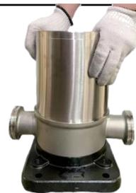
Fit and press the Cylinder (#55) firmly into place.
