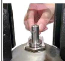
Install the shaft pin (#57)
